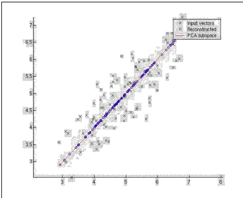
Principal Component Analysis used to find the 1D representation of the input 2D data with the minimal reconstruction error.
